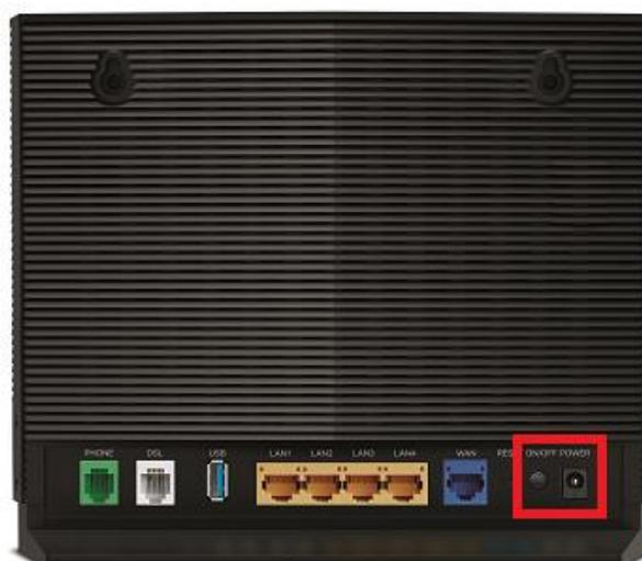
3. You can connect devices such as PC desktops, laptops or gaming consoles by plugging Ethernet cables from the devices to any of the **yellow LAN ports**, or you can connect devices via WiFi.
