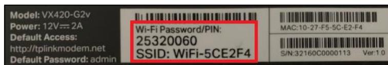
Your modem will automatically connect your devices to the best WiFi network possible (5Ghz). However, the older devices may only be capable of connecting to the 2.4Ghz WiFi network.
